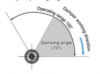
Right-handed: damper works when the shaft is turned clockwise (this figure) Left-handed: damper works when the shaft is turned counterclockwise (symmetrical to this figure)
